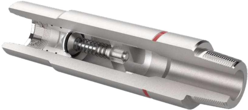
Float valve is a well control device protecting PDM from cuttings invasion during drill-string running. Float valve is installed above PDM. When used in combination with dump valve, float valve is installed below the dump valve.
