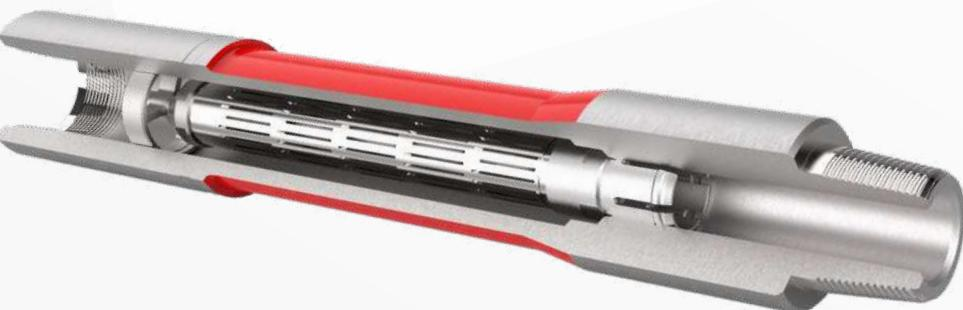
The main purpose of downhole motor filter is to protect motor, MWD and other BHA components from foreign particles damage. Filter is installed directly above the motor or MWD system.
