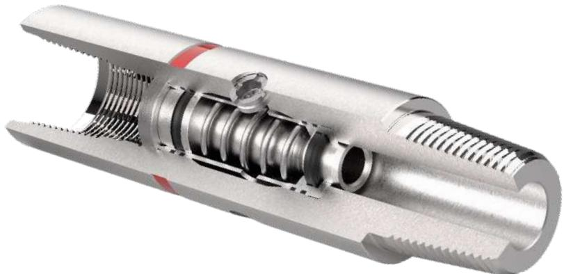
Dump valve is used for drill string filling and dumping during trips. Is installed above PDM. When used in combination with float valve, dump valve is installed above the float valve.
