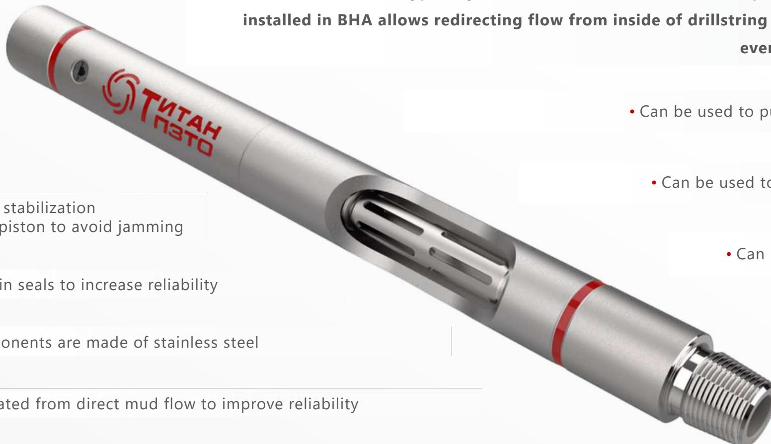
Circulation sub is a flow bypass system which can be activated multiple times. A simple tool installed in BHA allows redirecting flow from inside of drillstring to annulus bypassing everything what is below
